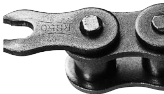
1) Static Fracture Stretching the link plate with a tensile load beyond its breaking load will cause it to stretch and then break.
